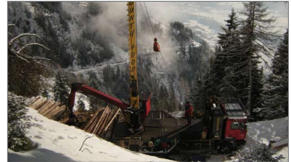
Deployment of a cable crane on a steep mountainside in Austria.
